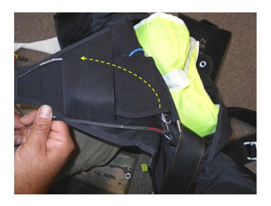
Pass the Ripcord cable and the Top Reserve Closing Flap under the T-IV retaining webbing.
