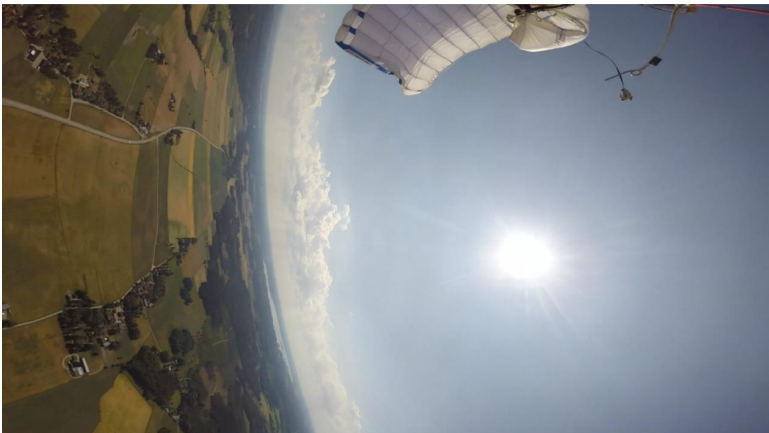
Picture 6. The main parachute with the Skyhook pulls the reserve pilot bridle. The Red Skyhook Lanyard is tense (upper right corner).
