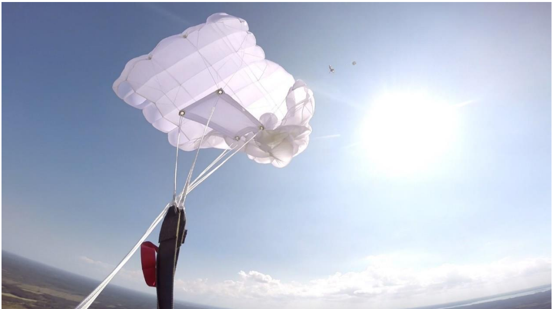
Picture 16. The reserve parachute immediately after opening. Above the reserve, the cut away main parachute and freebag. Note! Only the left risers are visible.
