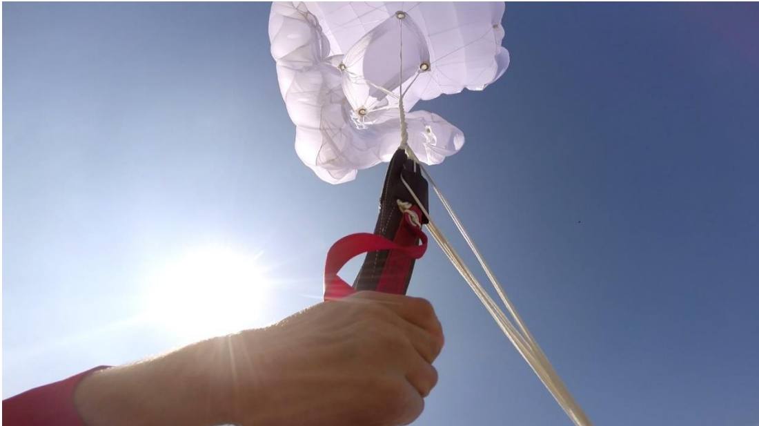
Picture 17. The reserve parachute incompletely developed and with line twists approx. 10 seconds after opening. Only the left risers are visible. The lines on the right side go down to the right risers below the image.
