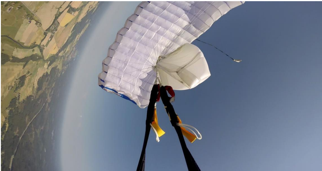
Picture 2. Main parachute with line twists approx. 10 seconds after pull.
