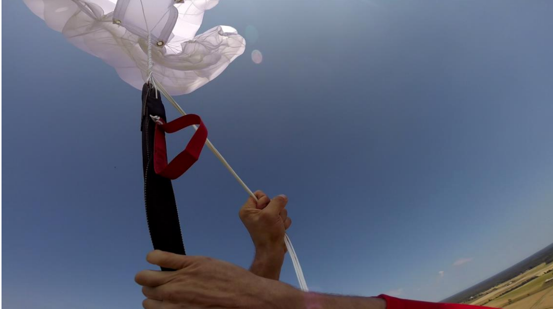
Picture 19. RB pulls the right suspension line group outwards and down.
