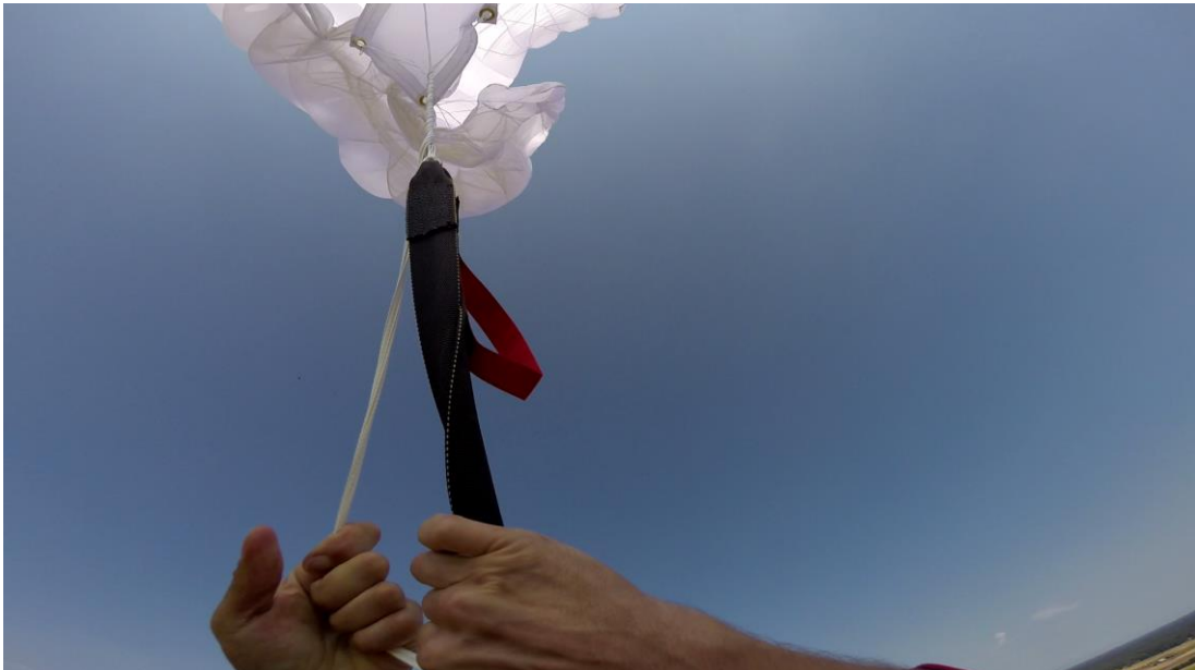
Picture 20. RB pulls the right suspension line group outwards and down.
