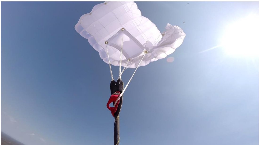
Picture 18. The reserve parachute with 3 cells out of 7 fully inflated.
