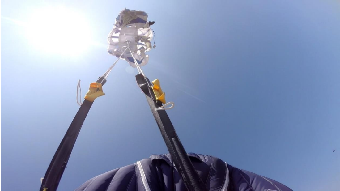
Picture 1. Main parachute with line twists immediately after the pull.
