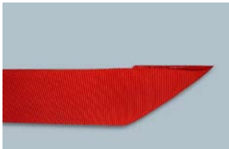
4.3 Prepare Tunnel with 25mm TYPE 3 Tape. Match size to Container
