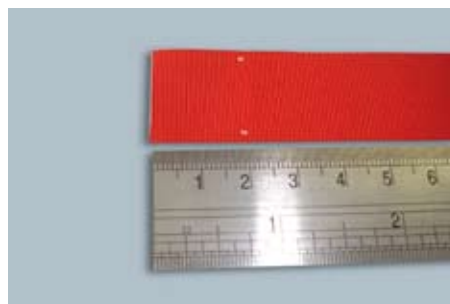
4.2 Measure and mark 20mm from Intersection between Flap #1 and Flap #2. This mark is the alignment mark for the start of the tunnel
