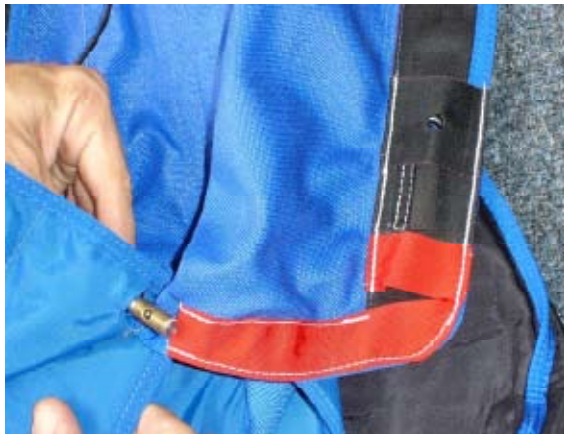
5.1 Thread Cutter thru slit in Panel #1
