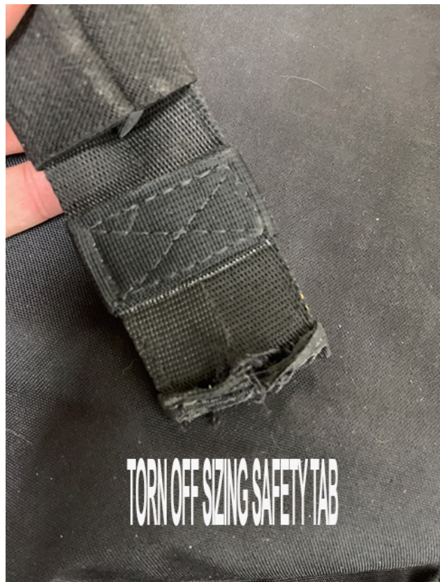
Torn off tab, damage free type 4
